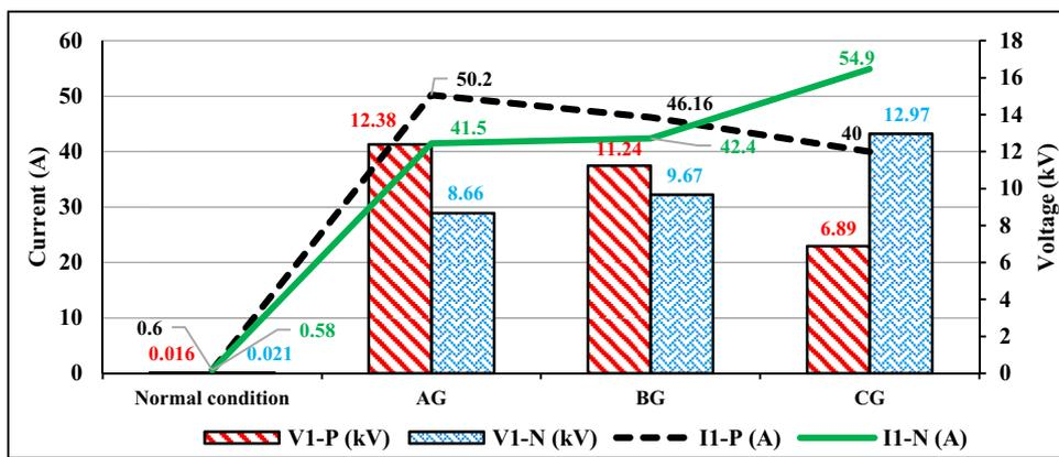
Fig. 6. Comparison diagram of induced fundamental frequency components in the positive and negative poles of the HVDC line for SLGF in different phases in the HVAC line compared to the normal condition.
