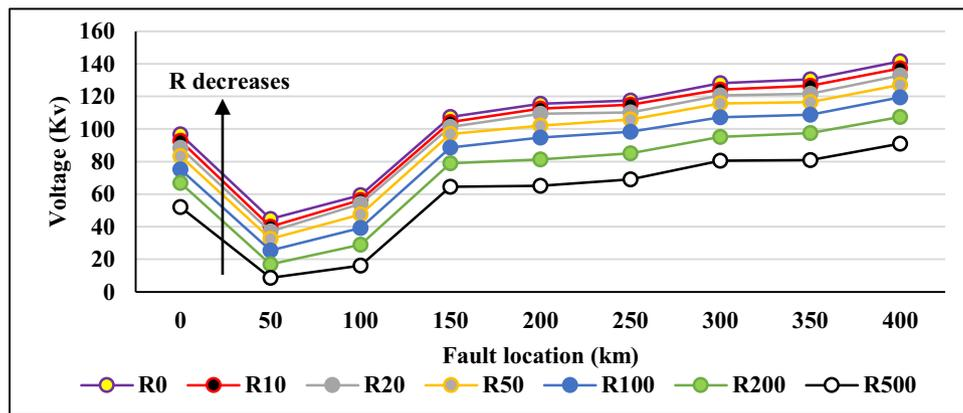
Fig. 12. Variations of fault location and fault resistance and its effect on the induced zero sequence voltage in the HVAC line for an SPGF in the “positive pole”.
