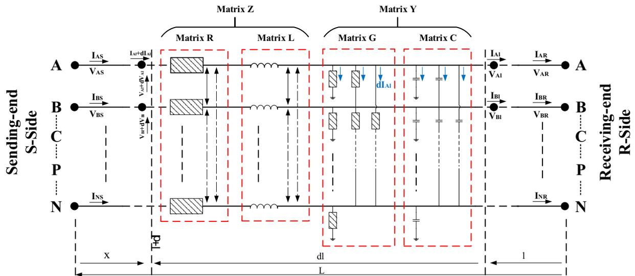
Fig. 3. The model used for extracting the equations of hybrid parallel transmission line.
