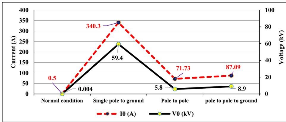
Fig 11. Comparison diagram of induced zero sequence components in the HVAC line at different DC faults condition compared to the normal condition.
