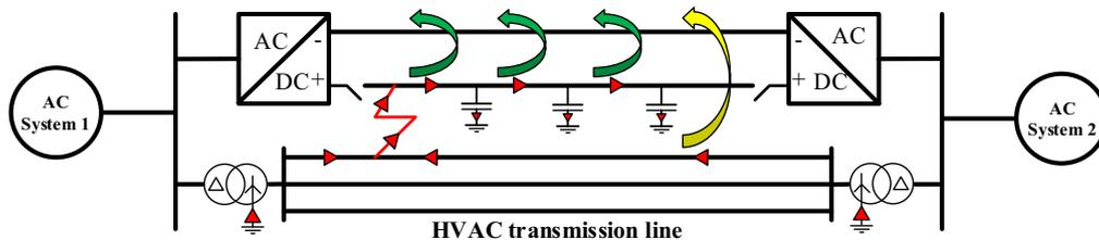
Fig. 16. Induced components under single pole (+) to phase "A" to ground fault.
