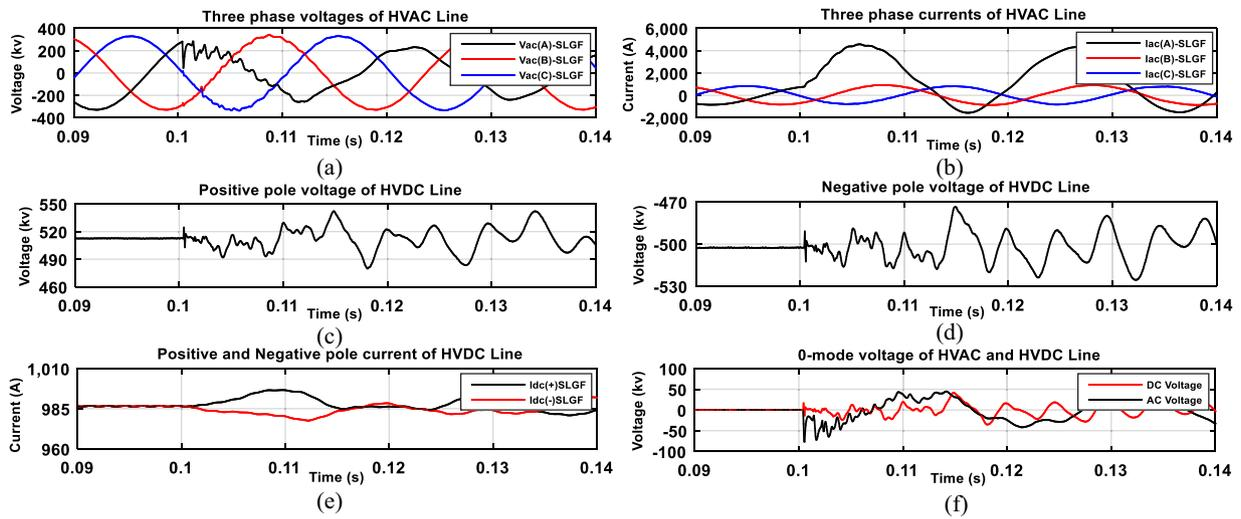
Fig. 4. AC and DC waveforms for an SLGF ("A" to ground fault) at  $x = 142$  km, a) AC line voltages, b) AC line currents and c) DC line positive pole voltage, d) DC line negative pole voltage, e) DC line currents and f) 0-mode voltage of AC and DC line.
