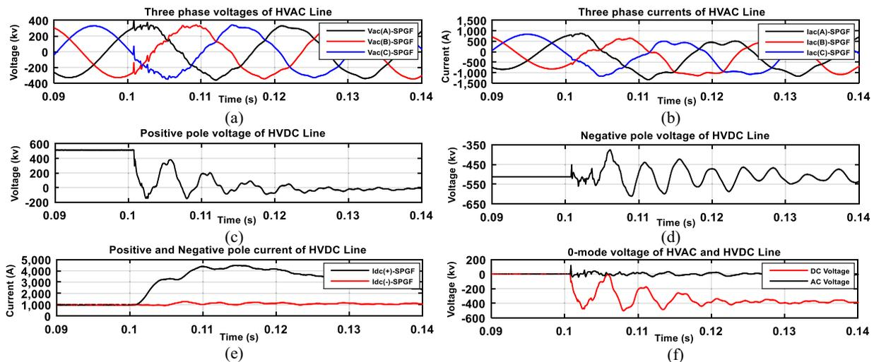
Fig. 10. AC and DC waveforms for SPGF at  $x = 264$  km, a) AC line voltages, b) AC line currents and c) DC line positive pole voltage, d) DC line negative pole voltage, e) DC line currents and f) 0-mode voltage of AC and DC line.
