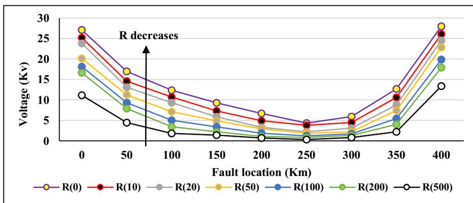
Fig. 7. Variations of fault location and fault resistance and its effect on the induced fundamental frequency voltage in the HVDC line (positive pole) for an SLGF in phase "A".
