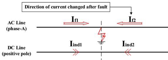
Fig. 9. Sign of the induced current and resulting inductive coupling during an SLGF.
