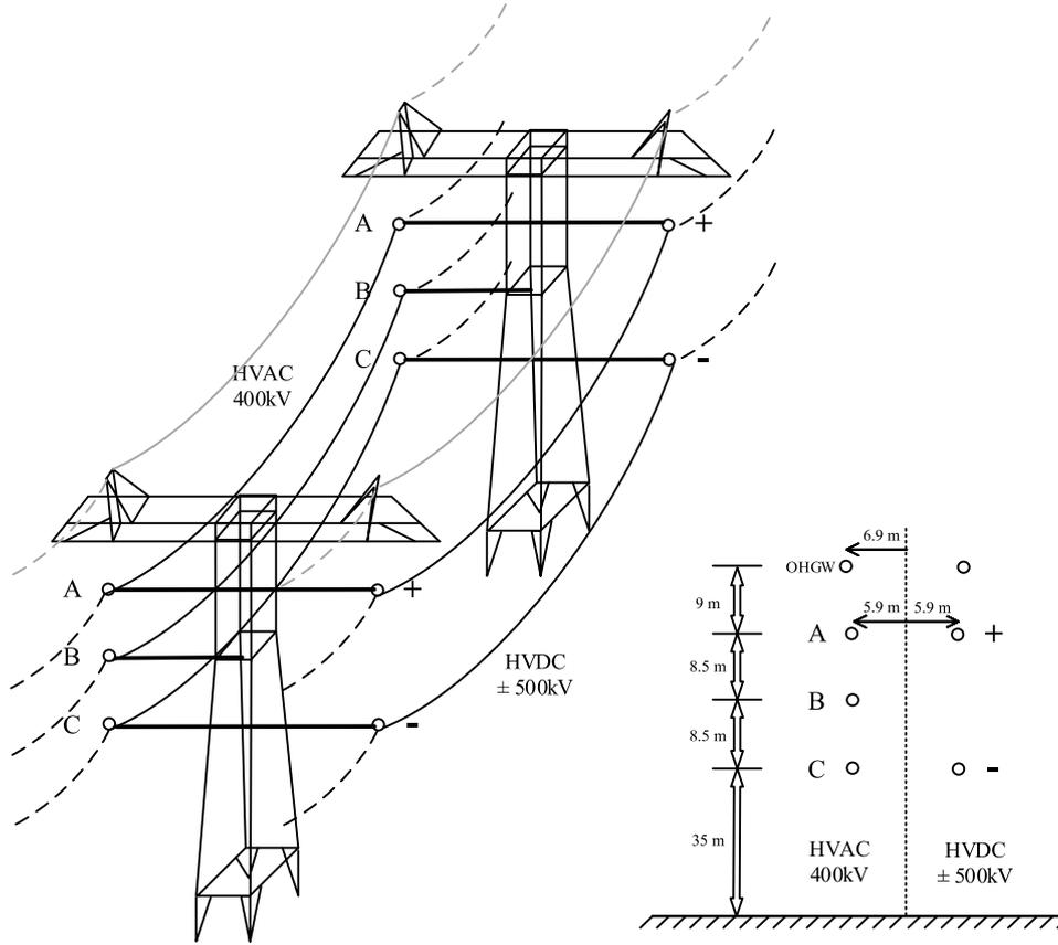
Fig. 2. Specifications of the HPOTL tower [21].
