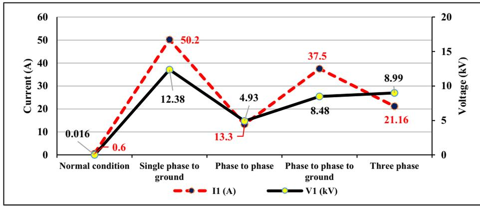
Fig. 5. Comparison diagram of induced fundamental frequency components in the positive pole of HVDC line at different AC fault conditions compared to the normal condition.
