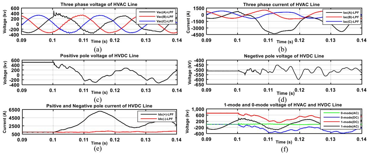
Fig. 15. AC and DC waveforms for LPF at  $x = 100$  km, a) AC line voltages, b) AC line currents and c) DC line positive pole voltage, d) DC line negative pole voltage, e) DC line currents and f) 1-mode and 0-mode voltage of AC and DC line.
