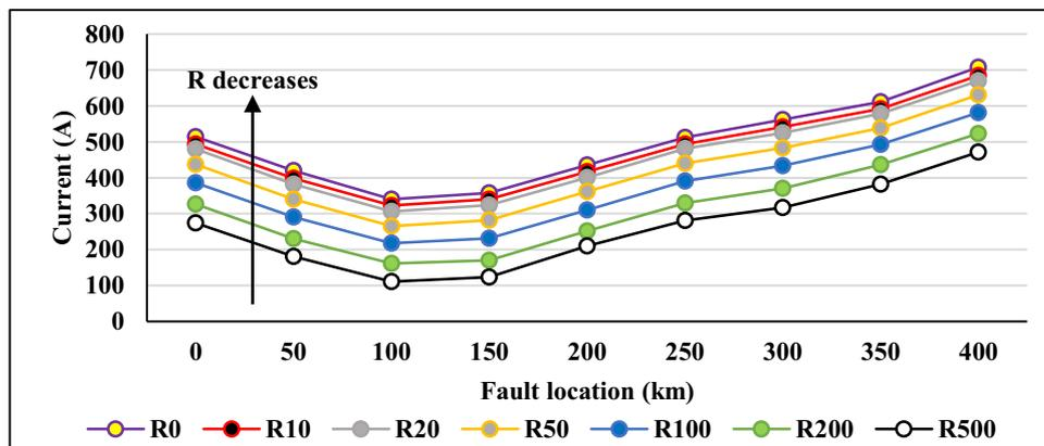
Fig. 13. Variations of fault location and fault resistance and its effect on the induced zero sequence current in the HVAC line for an SPGF in the “positive pole”.
