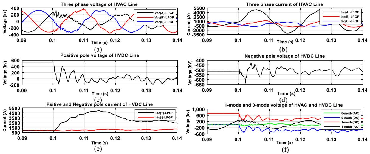
Fig. 14. AC and DC waveforms for LPGF at  $x = 100$  km, a) AC line voltages, b) AC line currents and c) DC line positive pole voltage, d) DC line negative pole voltage, e) DC line currents and f) 1-mode and 0-mode voltage of AC and DC line.
