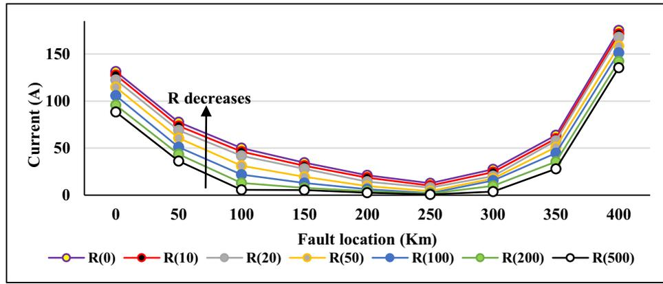
Fig. 8. Variations of fault location and fault resistance and its effect on the induced fundamental frequency current in the HVDC line (positive pole) for an SLGF in phase “A”.
