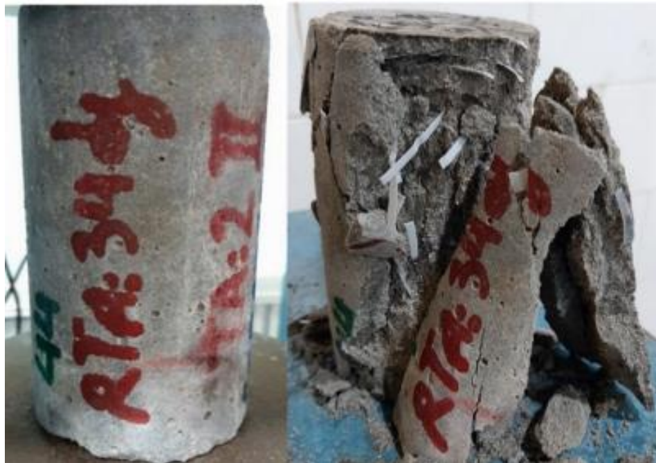
Figure 4. TA2: II and Retest 44-RTA2-II-S980722P7-34 after ultimate loading.
