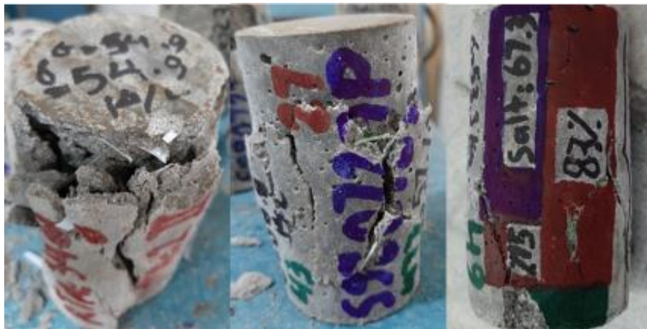
Figure 6. Plastic fiber behavior at a ratio of 83% Salt Water in cracking spread.
