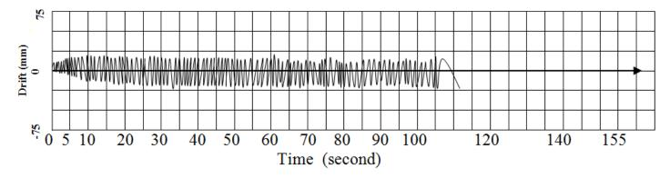
Figure 10. Drift with Respect to Time Under Cyclic Loading of GT-200 Panel.
