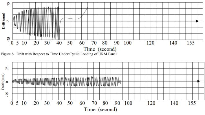
Figure 9. Drift with Respect to Time Under Cyclic Loading of GT-100 Panel.
