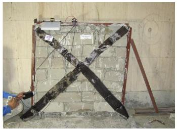
Figure 2. Test apparatus with CFRP applied to wall.
