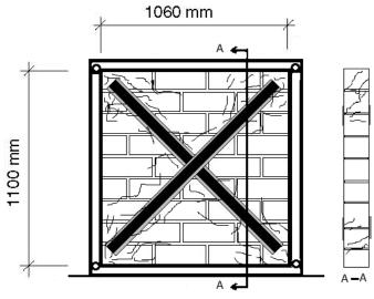
Figure 5. Corner Failure (CFRP-200-1).
