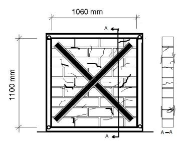
Figure 6. Splitting Crack and Delamination (CFRP-200-2).
