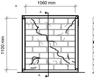
Figure 3. Splitting Crack (URM-1).
