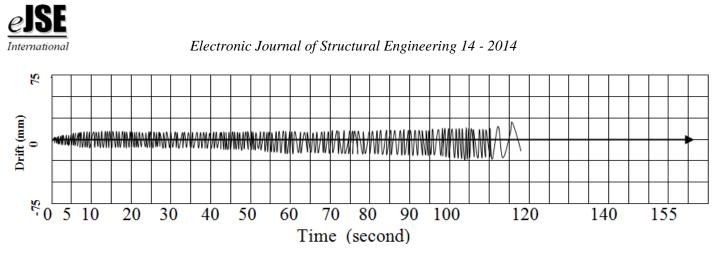
Figure 11. Drift with Respect to Time Under Cyclic Loading of CFRP-100 Panel.
