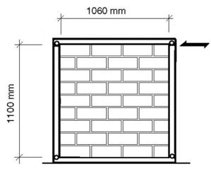
Figure 1. Idealized test arrangement.
