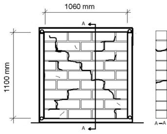
Figure 4. Horizontal Mortar and Splitting Crack (URM-2).
