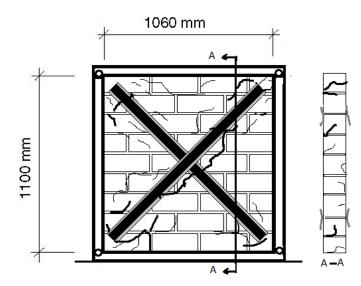
Figure 7. Corner Failure and Delamination (GT-200-2).
