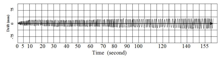
Figure 12. Drift with Respect to Time Under Cyclic Loading of CFRP-200 Panel.
