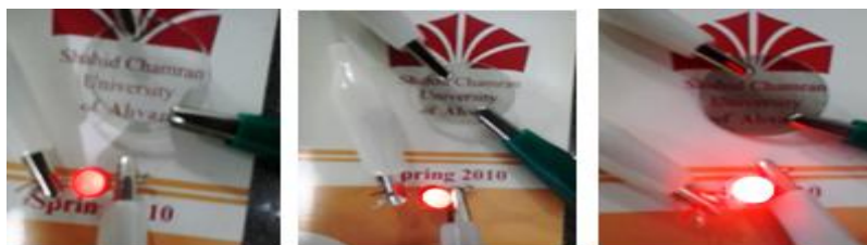
Fig. 2. Transparency of the films with circuit set up to light an LED, using the films in series with a battery.
