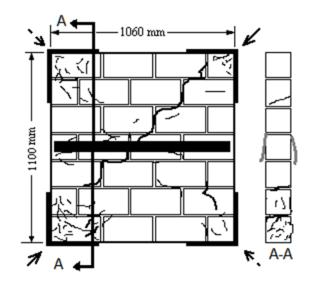
Figure 19. Cracking of CHF1.
