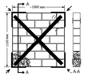
Figure 17. Cracking of CDF1.
