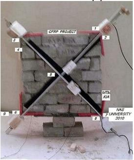
Figure 9. Test Setup for Cyclic Loading Tests. (Key: 1, 3, 7 and 9 are hydraulic rams, 5 is tension rods, 2, 4, 6 and 8 are seats on the edges.)
