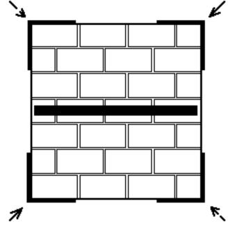
Figure 7. Test arrangement for horizontally reinforced panels under cyclic loading (CH).
