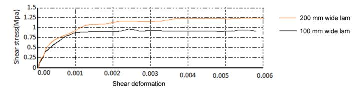
Figure 11. Response of Average of MDL3 and MDL4 in red and MDL1 and MDL2 in black.
