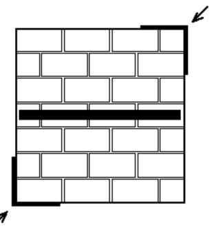
Figure 5. Test arrangement for horizontally reinforced panels under monotonic (MH).
