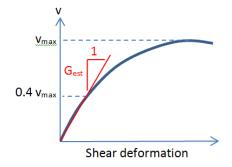
Figure 24. Method of calculation of monotonic shear modulus.
