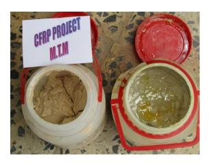
Figure 3. Kimitech Epoxy components (EP-TX).
