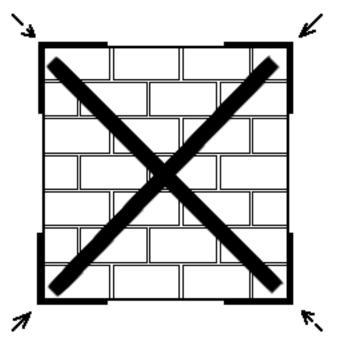
Figure 8. Test arrangement for diagonally reinforced panels under cyclic loading (CD).
