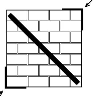
Figure 6. Test arrangement for diagonally reinforced panels under monotonic loading (MD).
