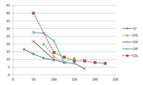
Figure 26. Equivalent Damping Coefficient at Various Load Levels (KN). Dashed are from Santa-Maria et. al. (2004).
