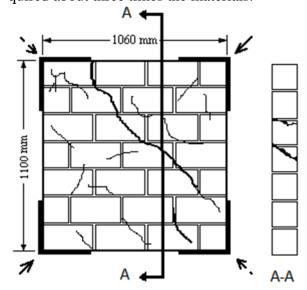
Figure 14. Cracking of CU1.
