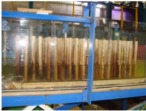
Fig. (3): Installation of cylindrical obstacles on experimental flume
